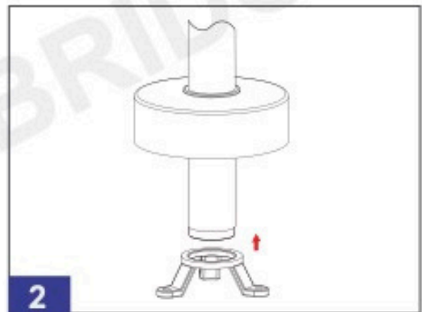
Step 2: Thread the tube onto the mounting tripod.
